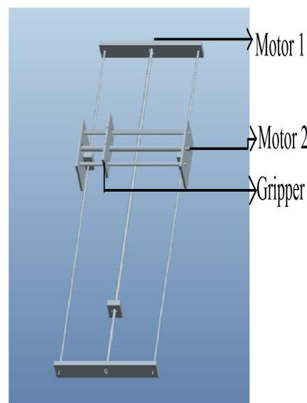
Fig. 2 CAD model of XY Table
