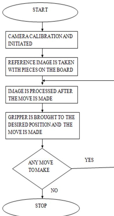
Fig. 3 Flowchart of the process
