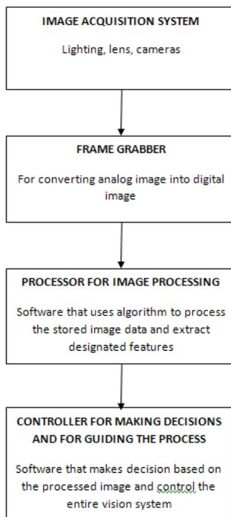
Fig. 1 Anatomy of a Machine Vision System
