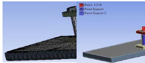
(a) Meshed model of existing Model (b) Loading and Boundary conditions of existing model
