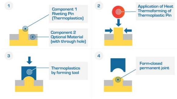
Figure 1: Heat Stacking Process
