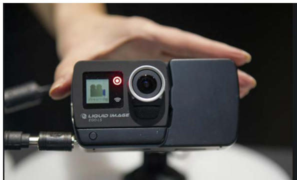
Fig 18 : A- Liquid Image wearable camera is paired with a 4G LTE. The camera and module combination make it the first wearable camera that can stream over LTE.
