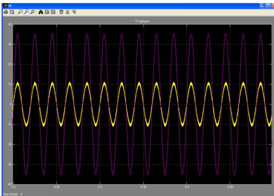
Fig.8. Supply voltage and current in phase
