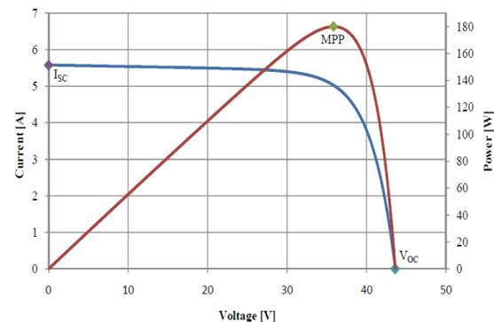
Fig.2 I-V and PV characteristics of PV cell
