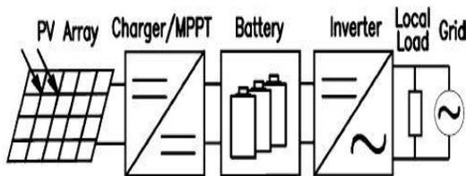
Fig.3 PV connected system
