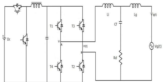
Fig5: Power stage circuit configuration single phase PV full-bridge inverter.
