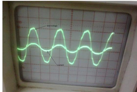
Fig.11 Inverter voltage and grid voltage before and after synchronized to grid
