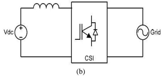
Fig.4 Simplify converter topology of grid-connected
