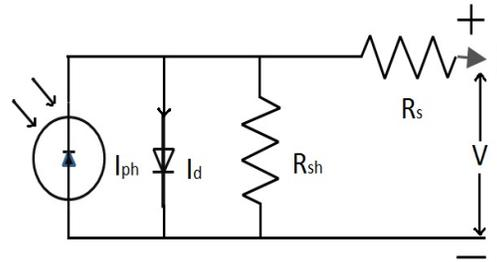
Fig. 1 equivalent circuit of PV
