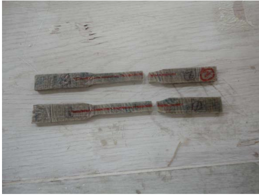
Fig: 4.Composite shaft after test
