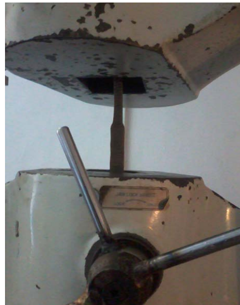
Fig: 3. Specimen in UTM Test Rig
