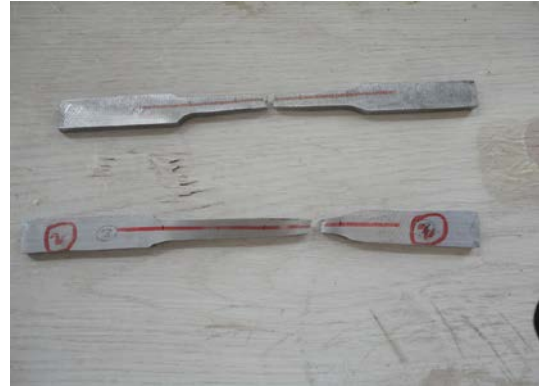
Fig: 5. Mild steel shaft after test
