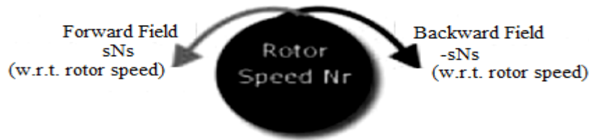
Fig.9 shows the Illustration of forward and backward rotating magnetic fields from rotor currents when a Broken Bar exists.
