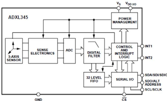
Fig. 2. Functional - Block Diagram of AD XL345
