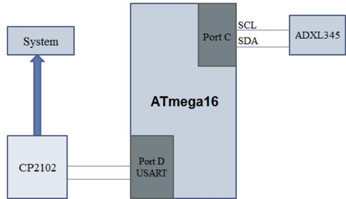
Fig. 4 . Hardware Inter Connection
