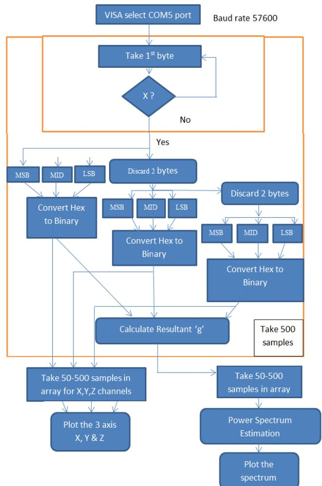
Fig. 7. Flow chart for Simulation in LabVIEW
