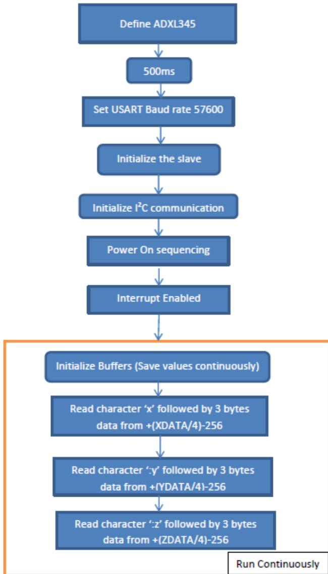
Fig. 6. Flow chart for ATmega I<sup>2</sup>C Communication with ADXL345
