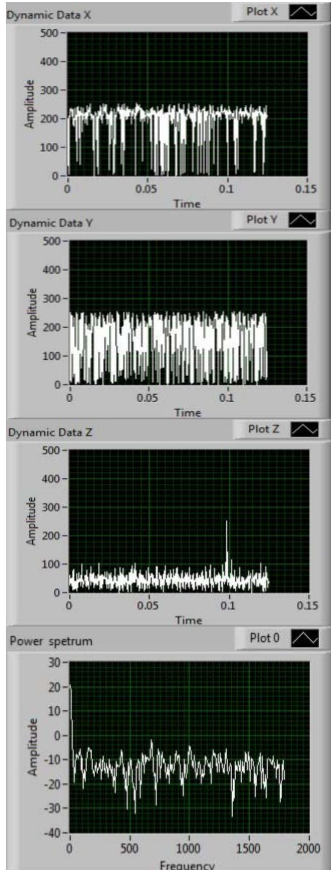
Fig. 9. LabVIEW output of ADXL345 when mounded on a motor of 3600rpm
