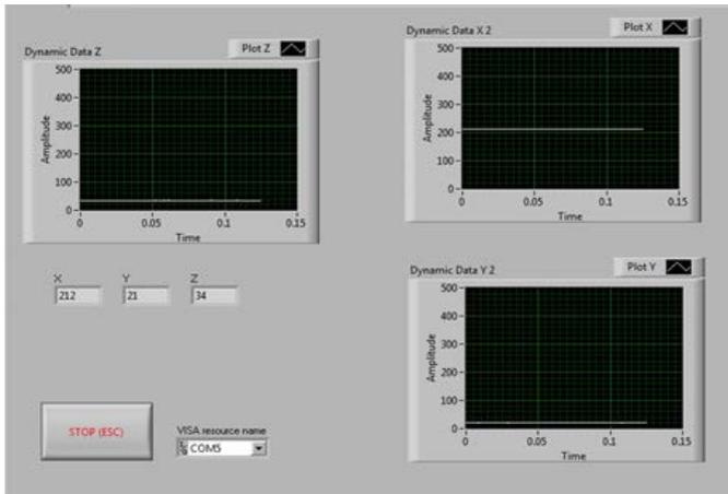
Fig 8. LabVIEW output of ADXL345 with no vibration input
