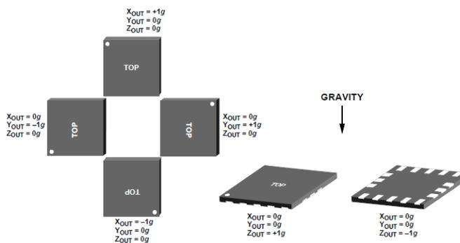
Fig. 3. Orientation towards gravity
