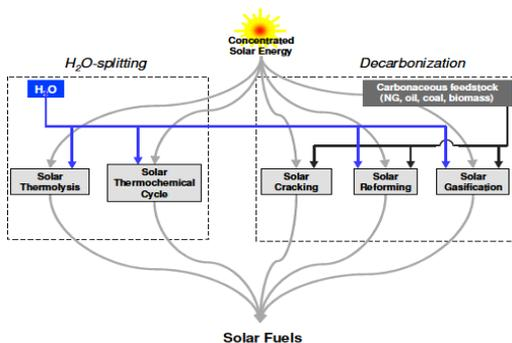
Five thermochemical routes for solar fuels production using concentrated solar radiation as the energy source of high-temperature process heat
