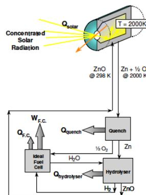
Schematic of an ideal cyclic process for calculating the maximum solar-to-fuel energy conversion efficiency of the 2-step water-splitting cycle using  $ZnO/Zn$  redox reactions
