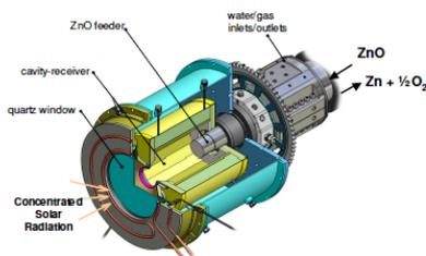
Scheme of the solar reactor configuration for the thermal dissociation of ZnO, as part of a 2-step water-splitting thermochemical cycle based on ZnO/Zn redox reactions. It consists of a windowed rotating cavity-receiver lined with ZnO particles. With this arrangement, ZnO is directly exposed to high-flux solar irradiation and serves simultaneously the functions of radiant absorber, thermal insulator, and chemical reactant
