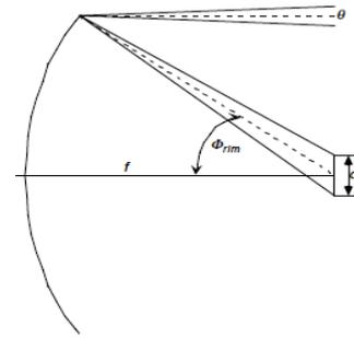
Figure 2. Concentration of sunlight by a parabolic dish of focal length  $f$  and rim angle  $\Phi_{rim}$ . When the dish is aligned toward the sun, reflection of sun rays at the focal plane forms a circular image centered at the focus of diameter  $d$ .
