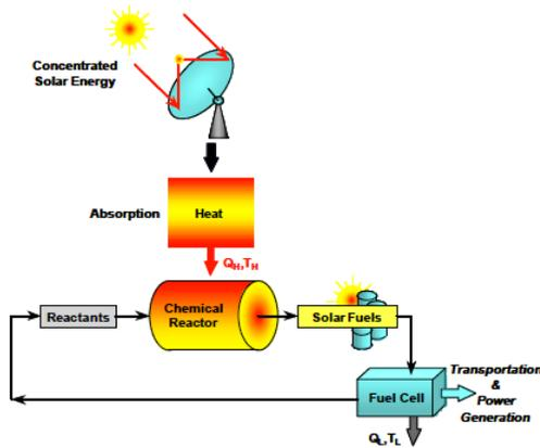
Figure 1. Schematic of solar energy conversion into solar fuels. Concentrated solar radiation is used as the energy source for high-temperature process heat to drive chemical reactions towards the production of storable and transportable fuels.
