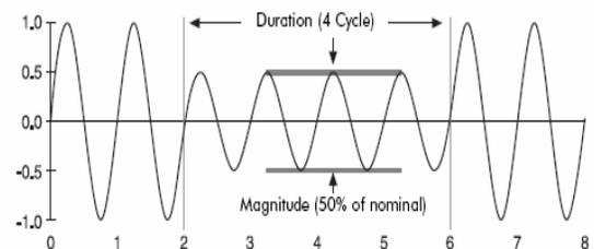
Fig.1. Voltage sag magnitude and duration
