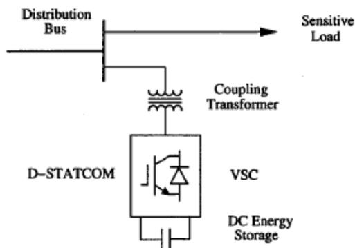
Fig. 4. . Schematic representation of the D-STATCOM as a custom power controller
