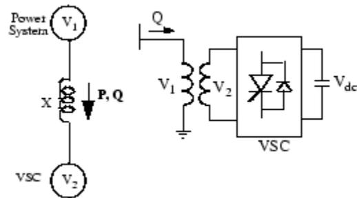
Fig.3 Configuration of STATCOM
