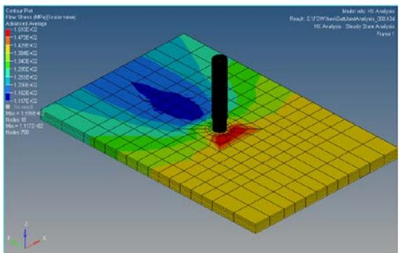
Fig-9. Flow stress distribution using Hexagonal Pin
