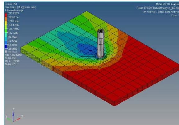
Fig-11. Flow stress distribution using Cylindrical Pin
