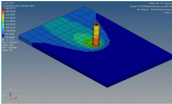
Fig-7. Temperature distribution using Cylindrical Pin
