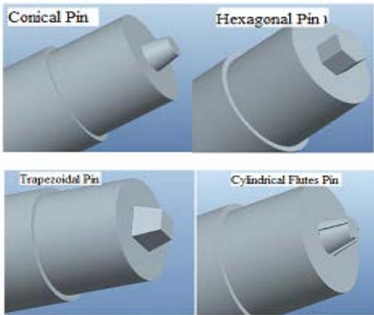
Fig.2. FSW Tools with different Tool-pin Profiles
