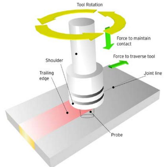
Fig.1 Schematic of Friction Stir Welding [2]
