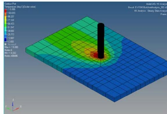
Fig- 4. Temperature distribution using Conical Pin
