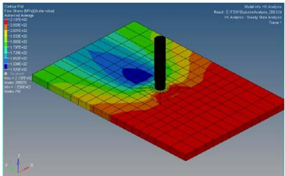
Fig-8. Flow stress distribution using Conical Pin
