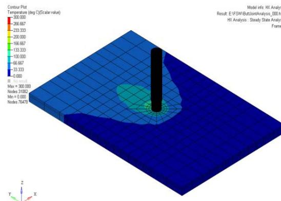
Fig-6. Temperature distribution using Trapezoidal Pin
