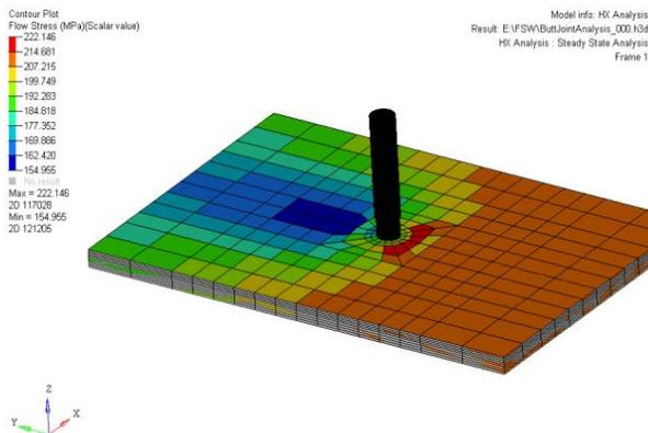
Fig-10. Flow stress distribution using Trapezoidal Pin
