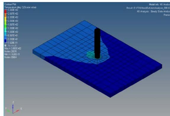
Fig-5. Temperature distribution using Hexagonal Pin
