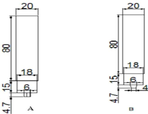
Figure.3 Tool Dimensions (a) With Hexagonal Pin
