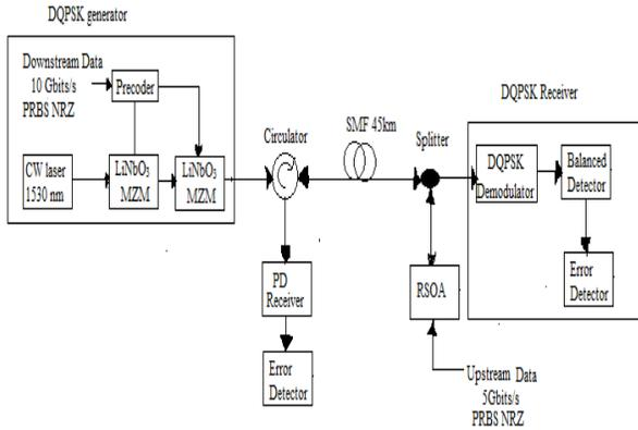
Fig. 2 Schematic diagram of a single channel bidirectional WDM system.
