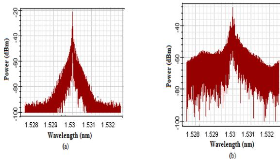
Fig. 3. Optical spectrum of (a) DQPSK and (b) re-modulated RSOA at frequency 1530nm.
