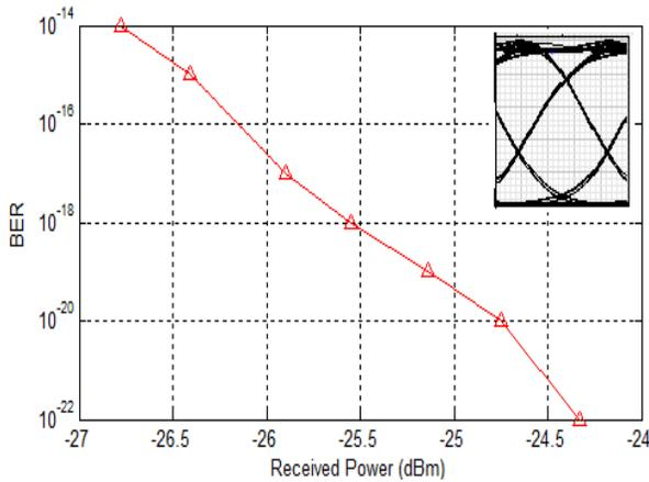
Fig. 6. BER vs Received curve of DQPSK is obtained at frequency 1530 nm.
