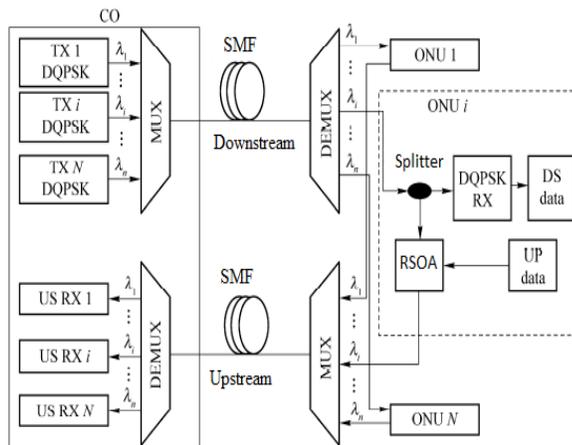
Fig. 1 The proposed Architecture of WDM-PON employing DQPSK downstream and OOK re-modulated upstream signals (DS/US: downstream/upstream)
