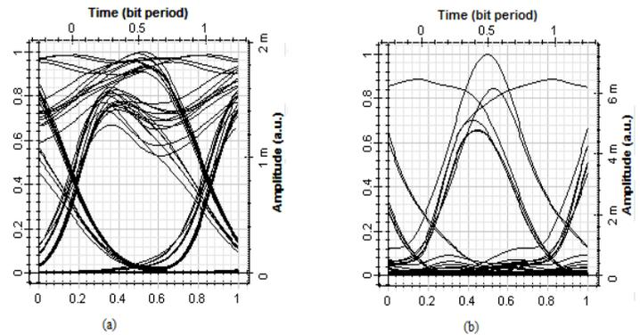
Fig. 4. Measured eye diagrams of upstream signal (a) re-modulated by RSOA with 0dBm CW light injection and (b) re-modulated by RSOA with 0dBm DQPSK modulated-light injection.
