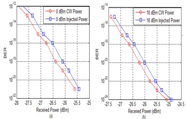
Fig. 5 (a) and (b). BER curve obtained at various optical powers incident on the RSOA.
