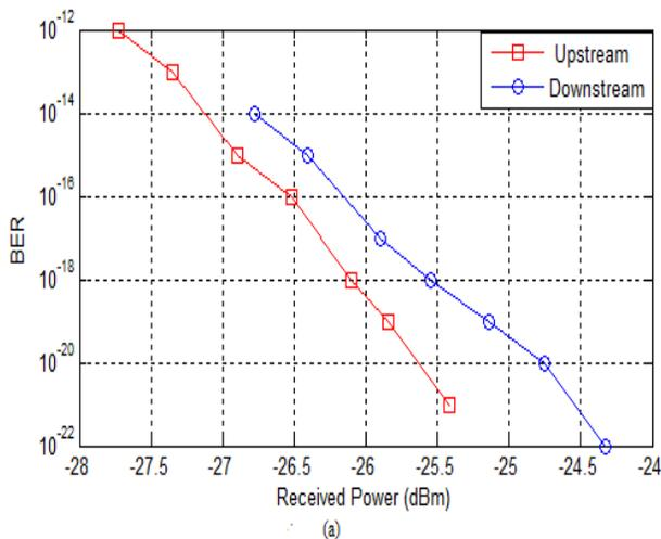
Fig. 7(a). BER vs Received power curves of downlink and upstream at input power 0dBm.
