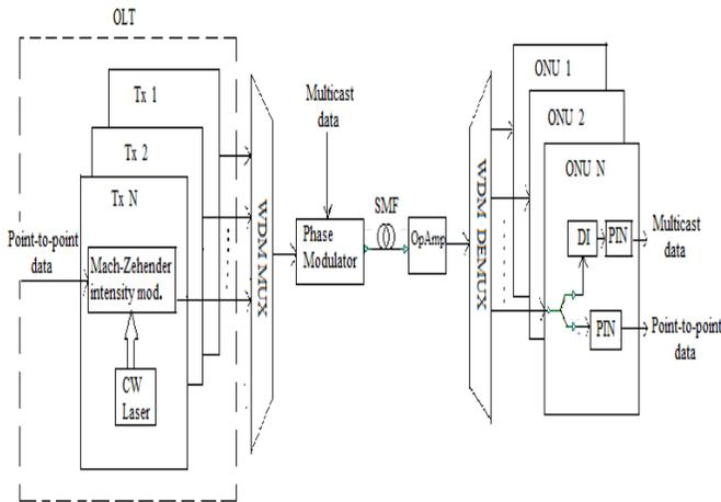
Fig. 1. Proposed WDM-PON architecture with multicast overlay.
