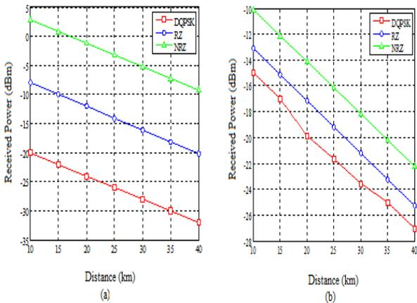
Fig. 4. Received Power v/s Distance measurements of all the three modulation formats with overlay of DPSK signal in case of (a) downstream signal at multicast, (b) downstream signal at point-to-point.
