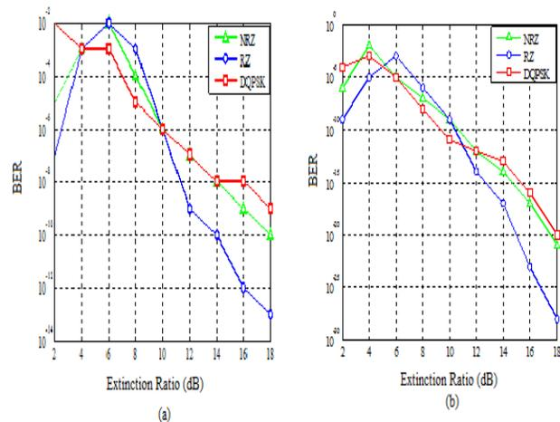
Fig. 5. Extinction Ratio v/s BER measurements of all the three modulation formats with overlay of DPSK signal in case of (a) downstream signal at multicast, (b) downstream signal at point-to-point.
