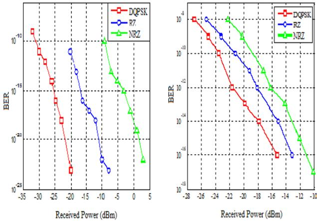
Fig. 3. BER v/s Received Power measurements of all the three modulation formats with overlay of DPSK signal in case of (a) downstream signal at multicast, (b) downstream signal at point-to-point.
