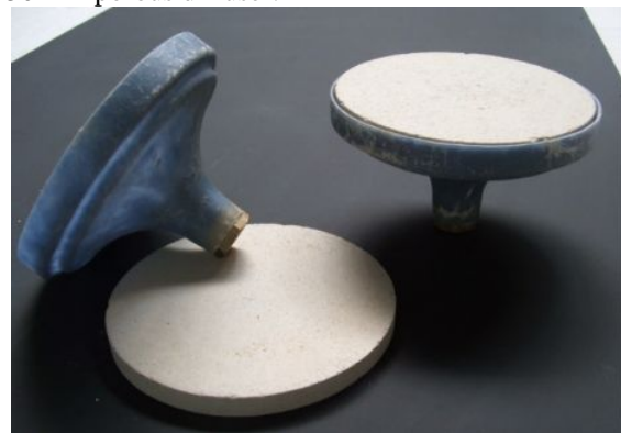
Fig. 1 Aspect of Ø150 ceramic porous diffusers.
