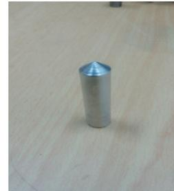
Fig.8- Aluminum pin locator.
