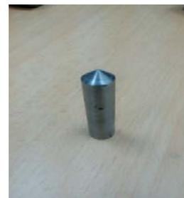
Fig.10- Mild steel pin locator.
