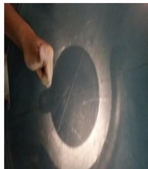
Fig.7-Piston surface check effect using P.Projector.
