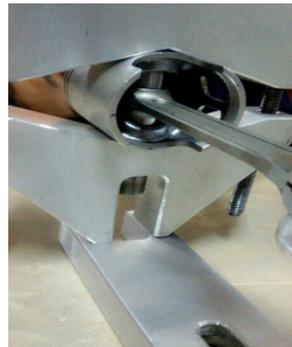
Fig.3- Pin Removal
