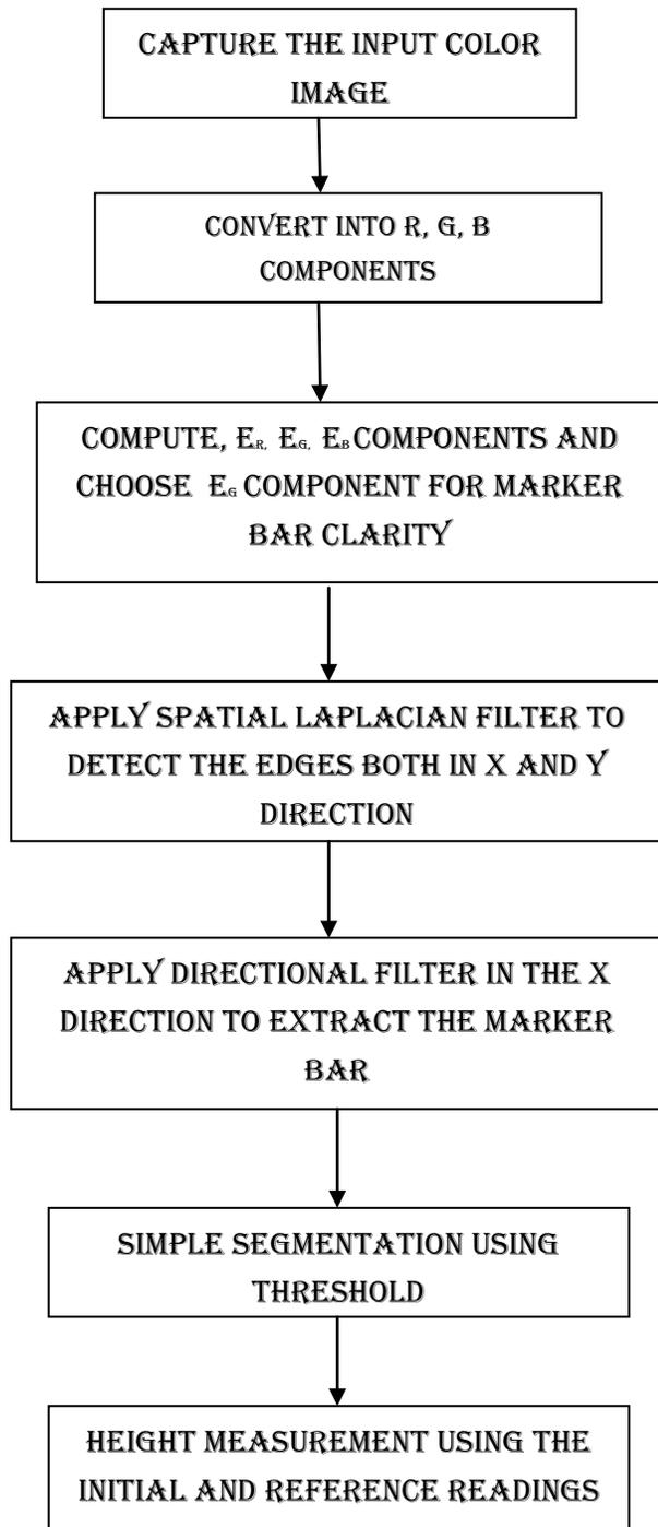
**Figure 1. Flow Chart for Height Measurement**
