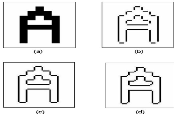
Figure.2. The comparison of the edge detections for the example image. (a) Original Image (b) Prewitt Edge Detection (c) Roberts Edge Detection (d) Sobel Edge Detection
