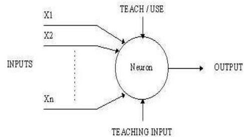
Figure.7. An artificial neuron with n inputs and one output
