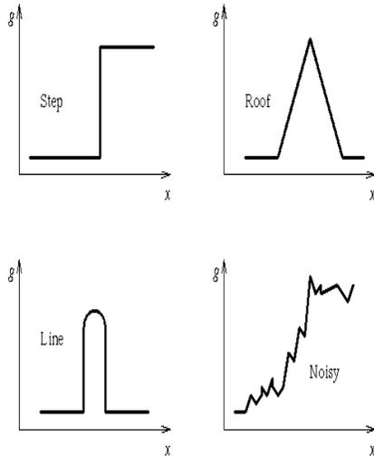
Fig 3.5 Typical edge profiles
