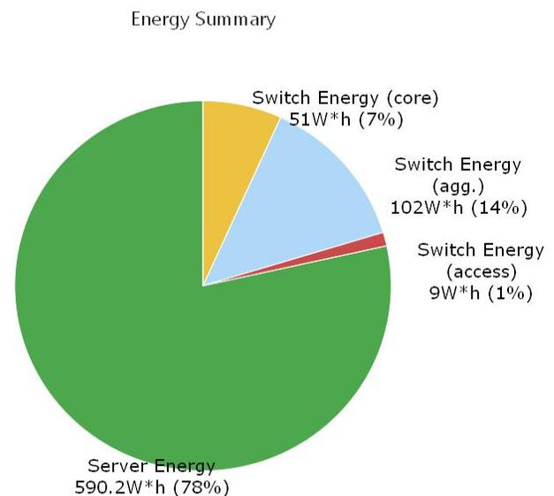
Fig.6. Distribution of Energy Consumption in a Data Center To incorporate the vast main stream of cloud computing applications, we define three sorts of jobs:
