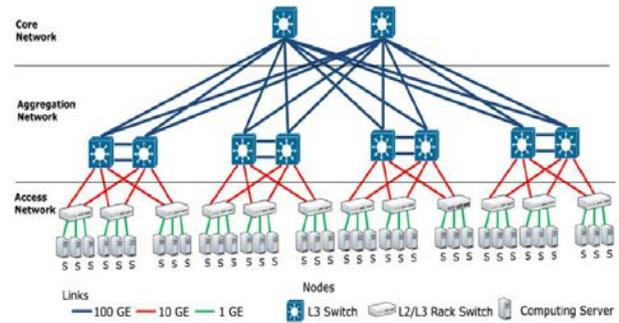
Fig.3 Three-tier high-speed Data Center Architecture
