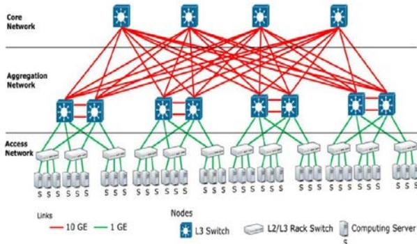
Fig.2 Three-tier structure in data center architecture
