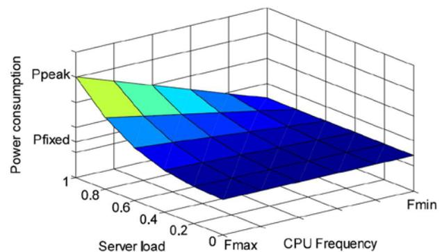
Fig.5 Computing Server Power Consumption
