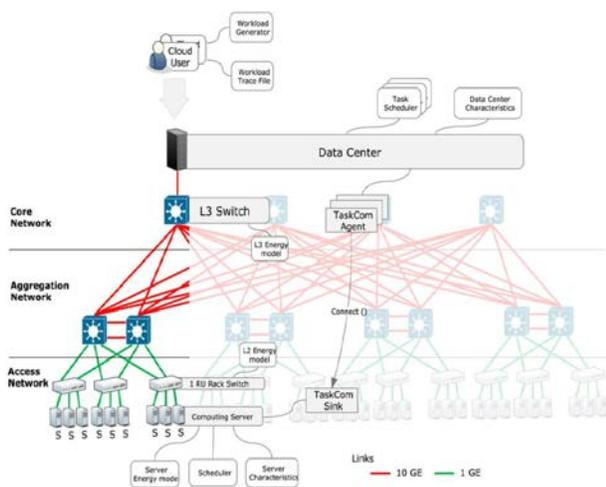
Fig.4 Architecture of the GreenCloud simulation environment
