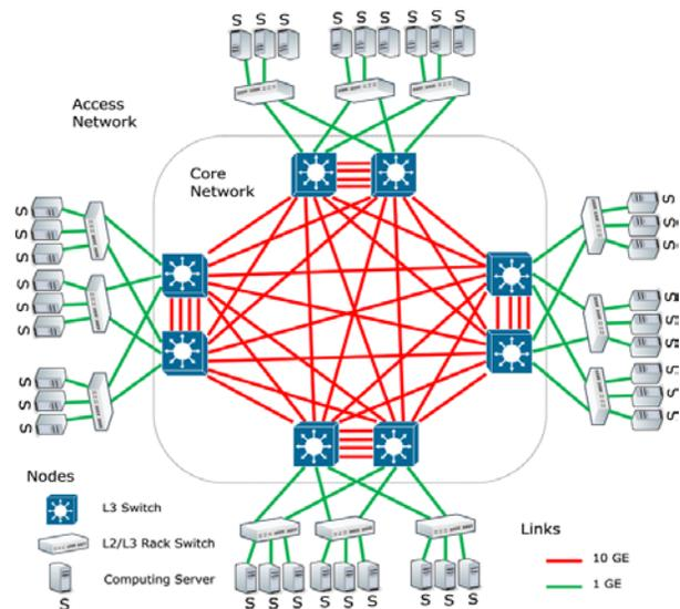
Fig.1 Two-tier structure in data center architecture
