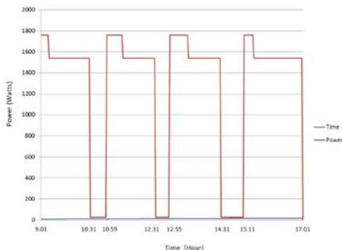
Fig 4 : Energy Consumption by the Existing system in a Working day
