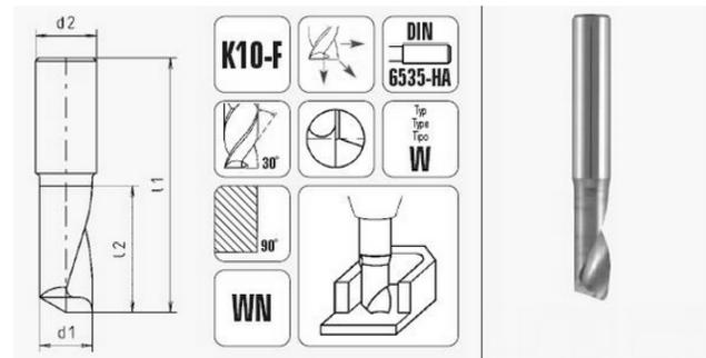
Fig. 1 Single flute end mill cutters - technical parameters [13]
