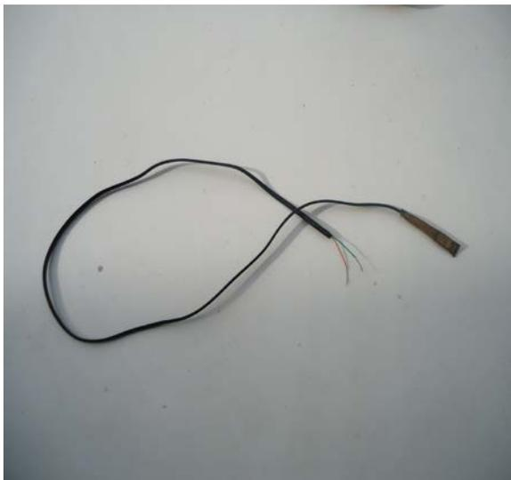
Fig. 2: Pictorial Diagram of a Thermistor
