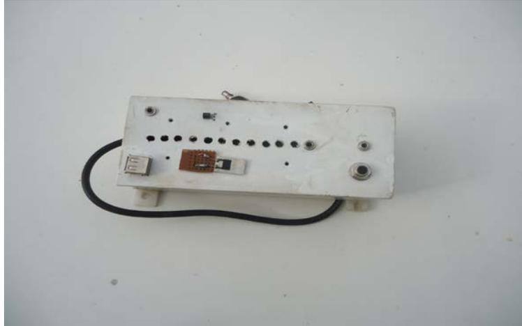
Fig. 4: Assembled data logger
