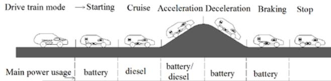
Fig. 2 Diesel hybrid vehicle movement
