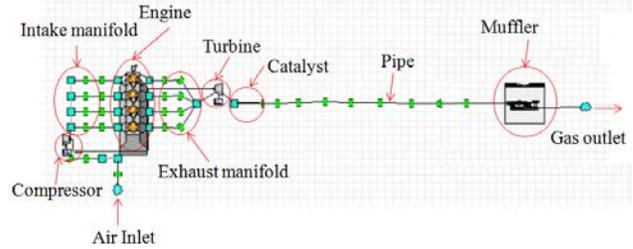
Fig. 7 Wave engine simulation model for 1.5l engine
