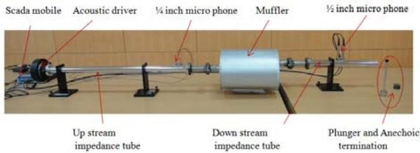
Fig. 15 Transmission loss measurement
