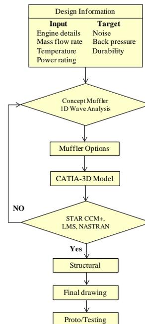
Fig. 5 Muffler design flow chart.
