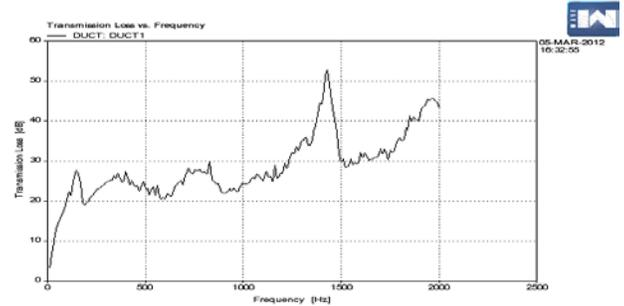
Fig. 12 Transmission loss Vs Frequency (1D)
