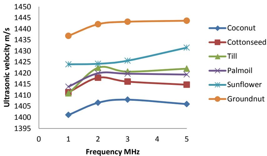
Fig 1. Ultrasonic velocity of various Vegetable Oils at vs Frequencies.
