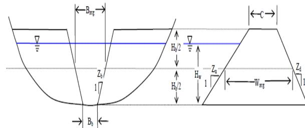
Figure 1. Breach describing parameters in the fracture of earth dams
