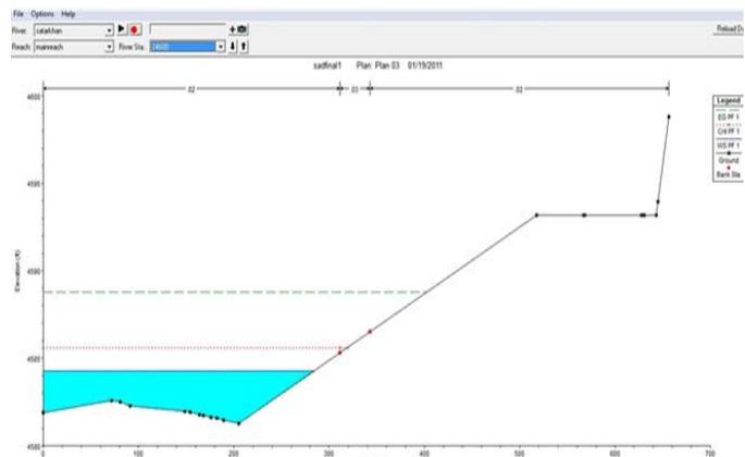
Figure5. the section of 24600 in dam fracture in Costa method
