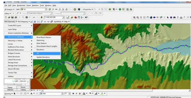
Figure2. presented river's cross sections and make them 3d by means of HEC GeoRas software
