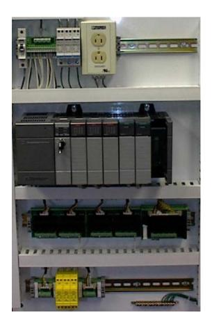
Fig: Control panel with PLC (grey elements in the center). The unit consists of separate elements, from left to right; power supply, controller, relay units for in- and output.
