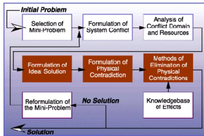
**Figure 2 Basic flow of problem reformulation using ARIZ**
