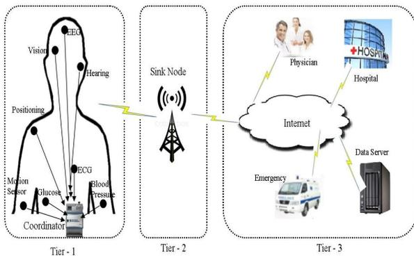
**Figure 2: Architecture of Wireless Body Sensor Networks**
