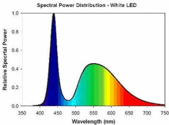
Fig. 2: Relative Spectral Power of Quasi-White LED. Source
