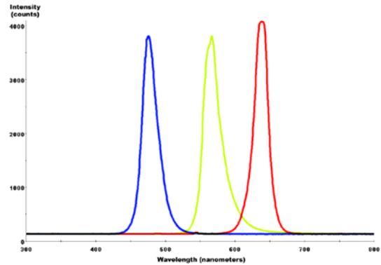
Fig. 3: Relative Spectral Power of RGB LED
