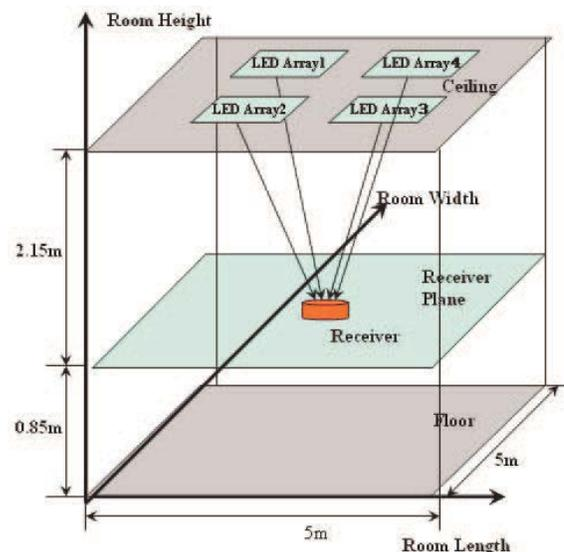
Fig.6: Typical VLC indoor lighting configuration
