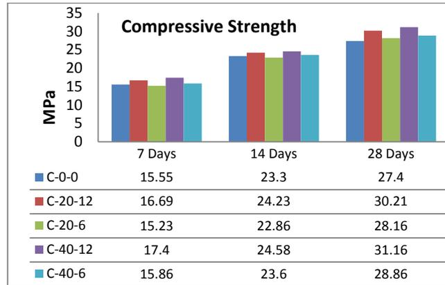
Figure 4- Graph of the results mean compressive test of 5 mix designs at different ages
