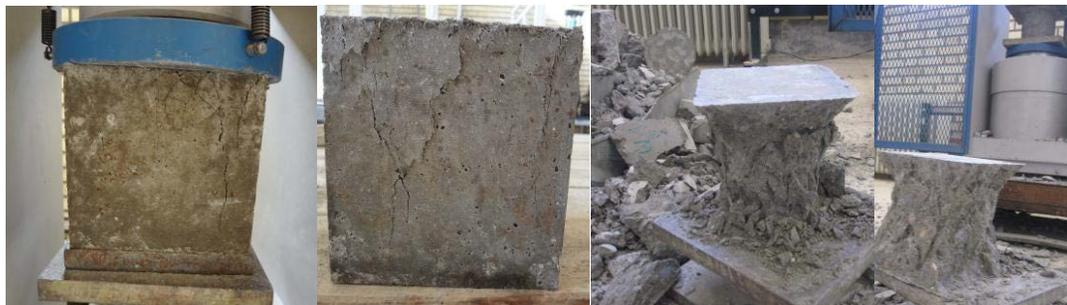
Figure 6- The failure of the concrete samples without fibers and with fibers at 28 days after the compressive loading
