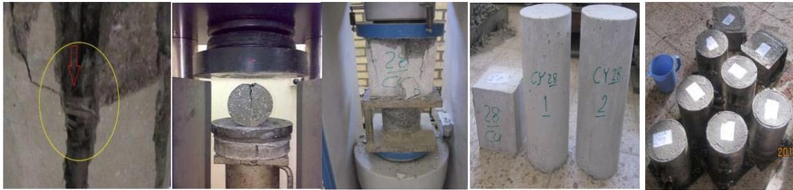
**Figure 3- Indirect Tensile strength and compressive strength tests for the sample C-20-12at 28 days after loading**
