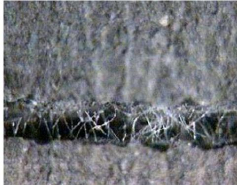
**Figure 7- Way of bridging fibers on the crack**
