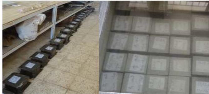
Figure 2- curing of concrete samples in the laboratory
