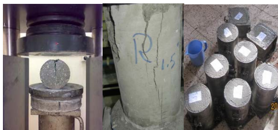
Fig. 1: Tests of indirect compressive and tensile strengths
