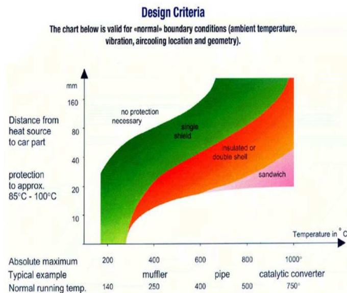
Fig2.1: Design criteria for heat shield.
