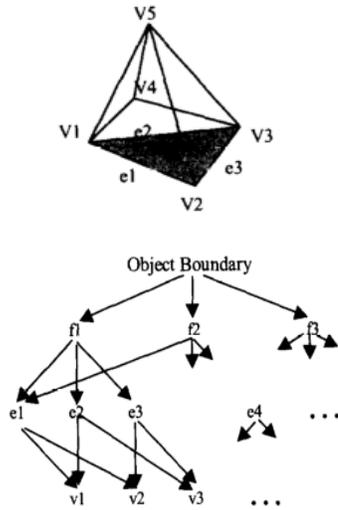
Fig 3: An example of boundary representation of a prism
