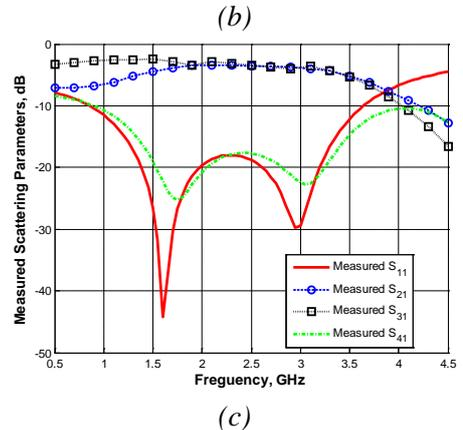
Fig. 2. (a) The proposed broadband branch-line coupler with L-shaped equivalent structure of the conventional transmission line. (b) Magnitude of Simulated scattering parameters (c) Magnitude of measured scattering parameters
