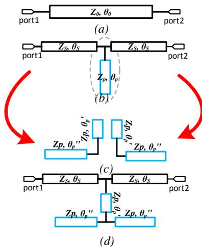
Fig. 1. (a) A conventional transmission line, (b)  $\pi$ -equivalent transmission line of the conventional type, (c) flipped vertically and folded equivalent structure of the open stub, and (d) H-shaped equivalent structure of the conventional transmission line.
