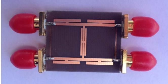
Fig. 3. photograph of fabricated coupler
