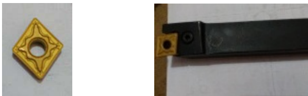
Fig: 2 carbide insert and seat clamp tool holder
