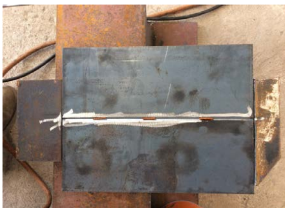
Fig. 1 Preparation of two plates for weld
