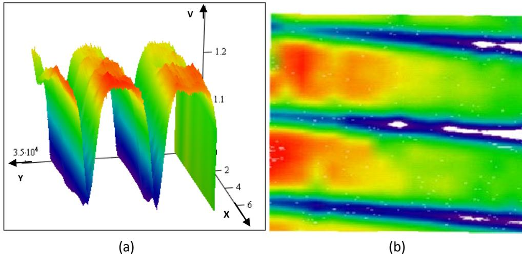
Fig. 9 a) 3-D surface plot of voltage generated against displacement as scanning is done in x and y direction (b) LBIV map as solar cell is scanned in x and y direction
