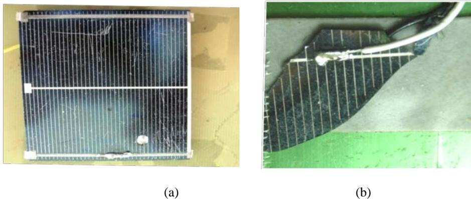
Fig. 1 (a) The delaminated solar cell from a crystalline module (b) A section of the delaminated cell cut and connected to the LBIC/LBIV
