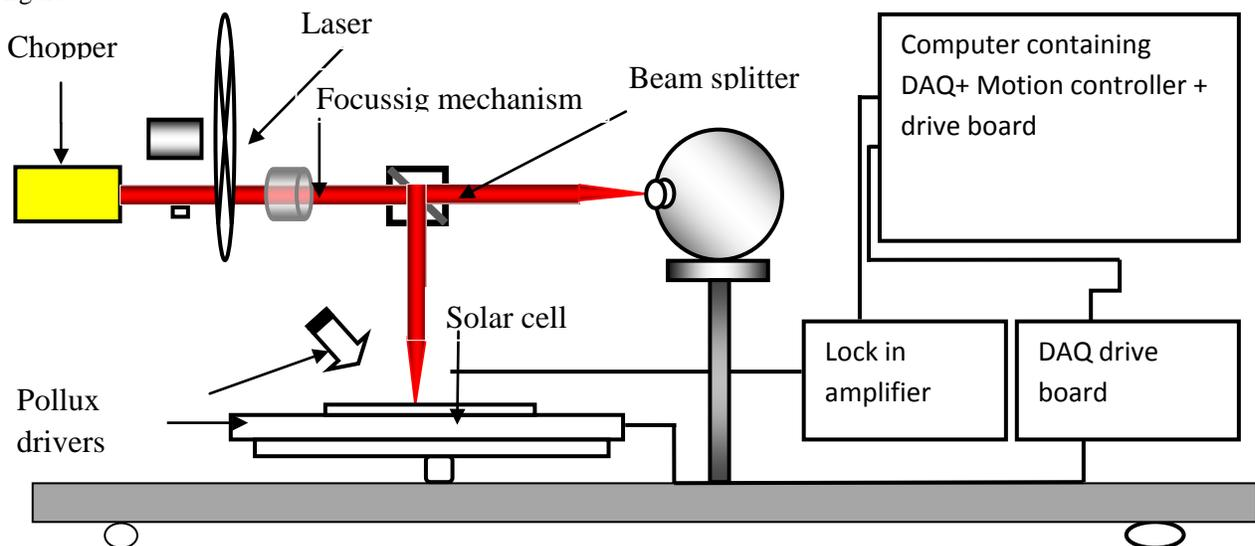
Fig. 3 The LBIC system design and construction with a laser beam falling on the surface of the solar cell <sup>[6]</sup>
