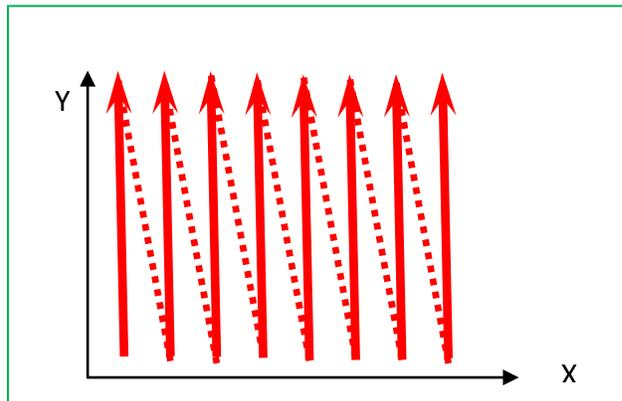
Fig. 2 Raster scan pattern used through the motion control.
