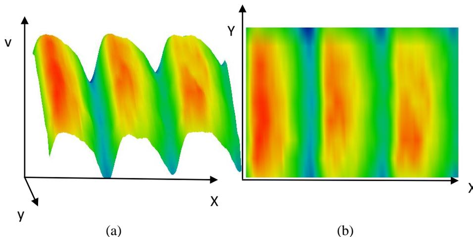
Fig. 8 (a) 3-D LBIV map for a mono-crystalline silicon solar cell voltage plot and (b) a rotated at different angle
