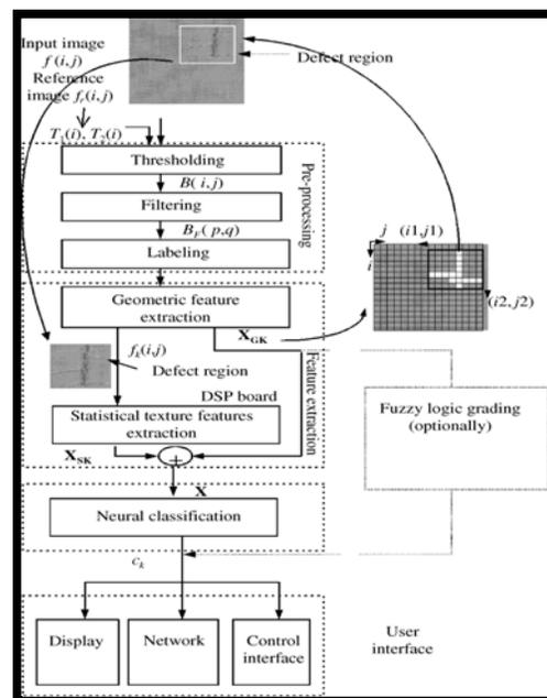
Fig. 5 Flow diagram of the proposed inspection algorithm [5]
