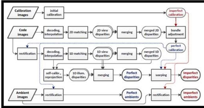
Fig. 3 Typical Software Processing Block Diagram [4]
