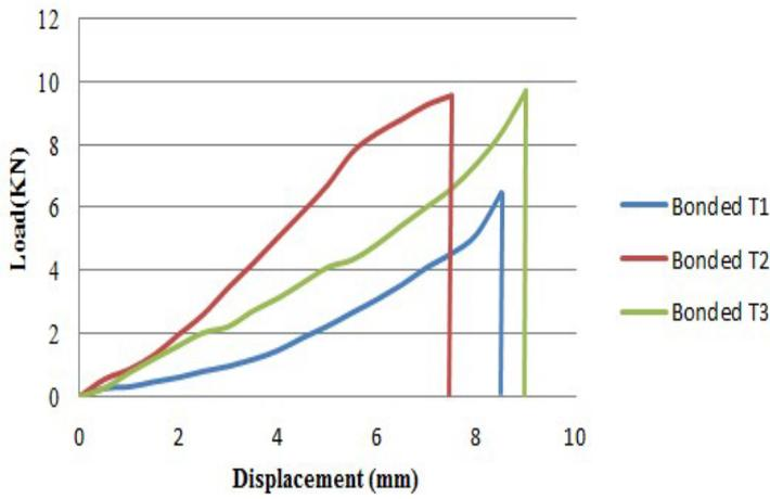
Fig.8 Graphs OF Load Vs Displacement Bonded Repaired Specimens.
