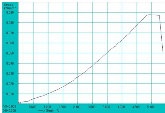
Fig.14 Stress Strain Ratio Of Bolted specimen.
