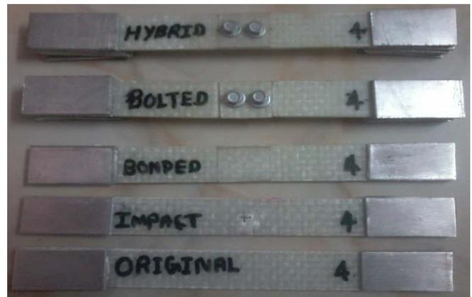
Fig. 3 Testing Specimens
