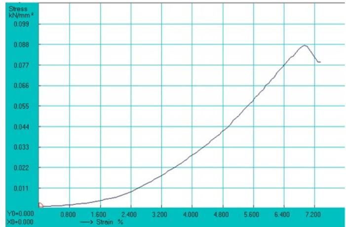
Fig.15 Stress Strain Ratio Of Hybrid Repaired specimen.
