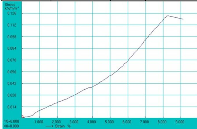
Fig.13 Stress Strain Ratio Of Bonded Repaired specimen.
