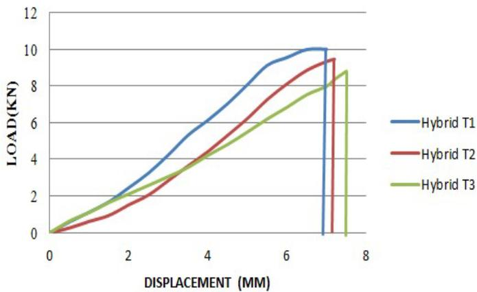
Fig.10 Graphs OF Load Vs Displacement Hybrid Repaired Specimens.
