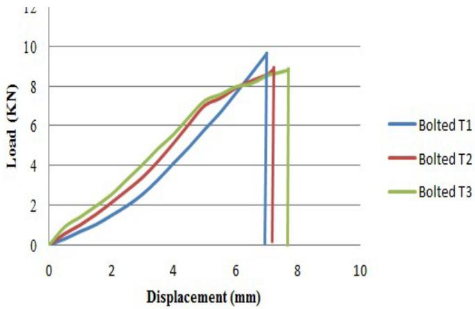
Fig.9 Graphs OF Load Vs Displacement Bolted Repaired Specimens.
