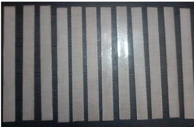
Fig. 1 ASTM D3039 Standard Specimens
