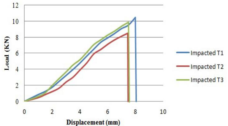
Fig.7 Graphs of Load Vs Displacement Impacted Specimen.
