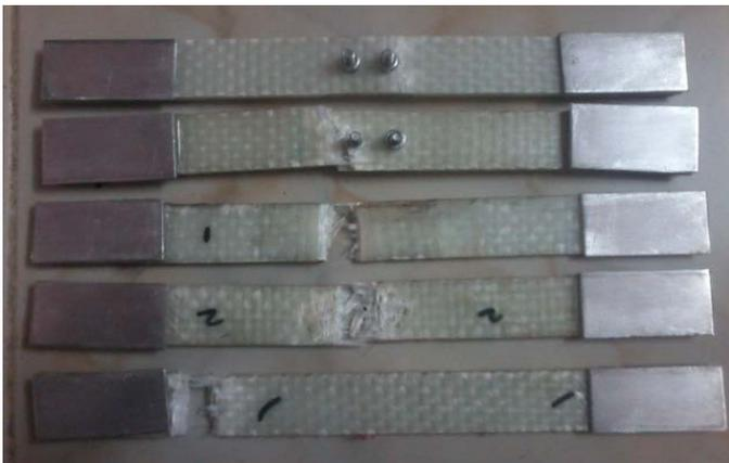
Fig.5 Tensile Test Of The Specimen.
