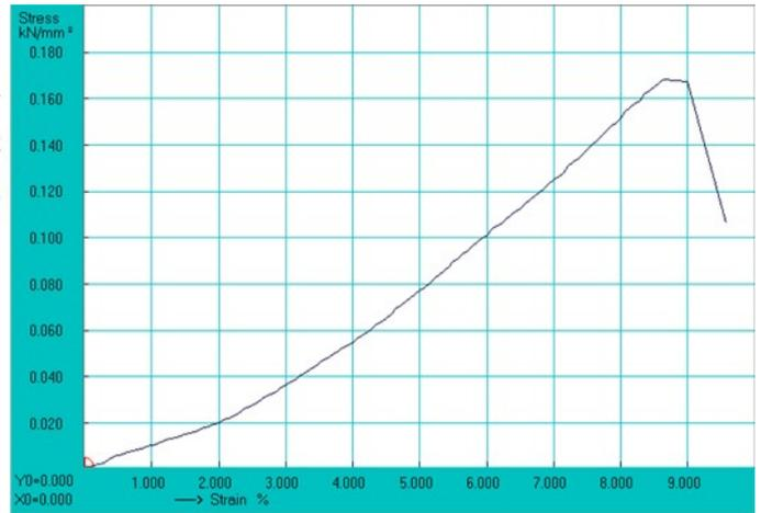
Fig.11 Stress Strain Ratio Of Original specimen.
