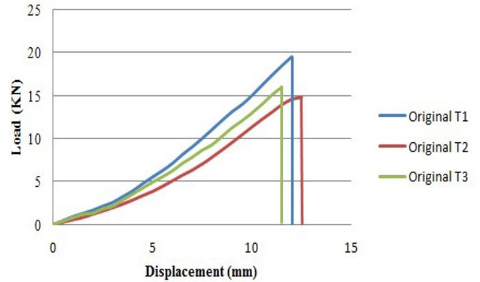
Fig.6 Graphs of Original Tensile Strength Of The Specimens.
