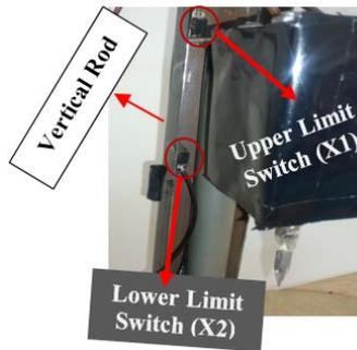
Fig. 5 Limit Switches Setup on the Project
