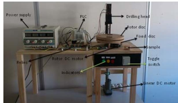
Fig. 1 Drilling System Prototype.
