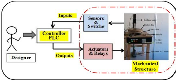
Fig. 2 Automated Drilling Machine System
