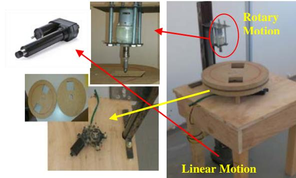
Fig. 7 DC Motors with Rotor and Linear Actuator.
