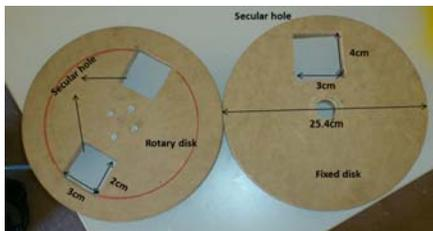
Fig. 11 Fixed and Rotary Disk
