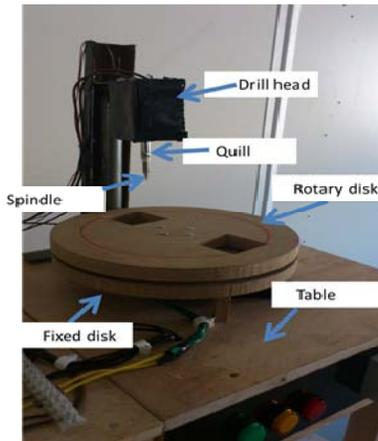
Fig. 10 Mechanical Structures of the project
