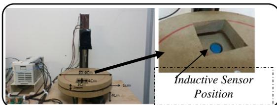
Fig. 3 Inductive Sensor Setup on the Project
