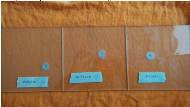
Figure 4: Specimen after machining 150 mm * 150 mm * 4 mm
