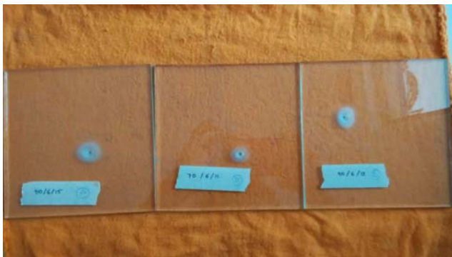
Figure 5: Specimen after machining 150 mm * 150 mm * 6 mm
