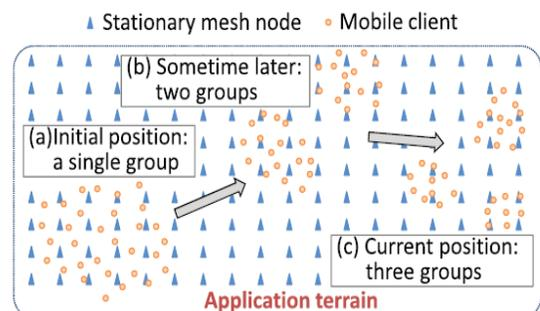
Fig. 2. Fixed grid-based square topology under three scenarios illustrated in Fig. 1.
