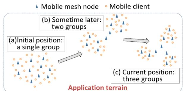
Fig. 1. Topology adaptation of the autonomous mobile mesh network under three scenarios.
