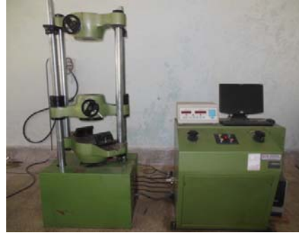
Fig4 Universal testing machine (model- MECH/UTE-40T).
