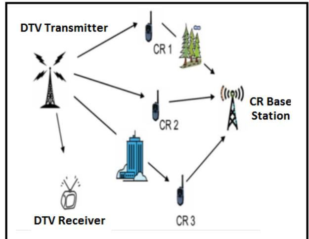
Fig.2 co-operative spectrum sensing in CR radio networks.
