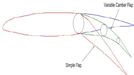
Fig: 2.1 Basic geometric design of the variable flap
