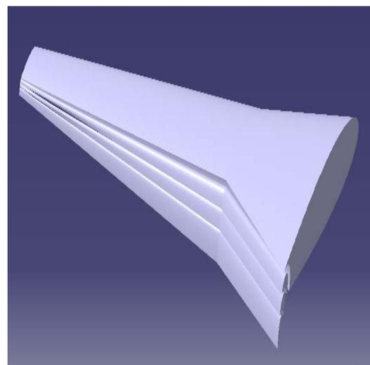
Fig: 5.1 Variable cambered wing model
