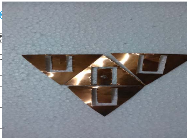
Fig. 4.10 Practical 4 U slotted antenna array
