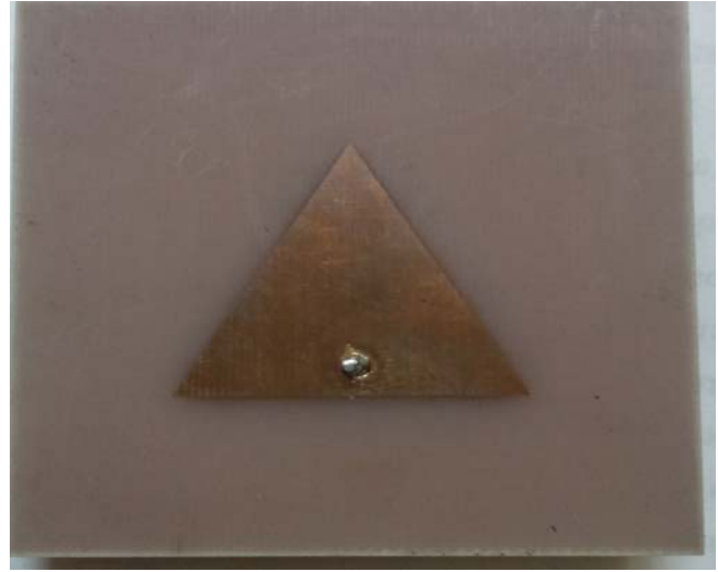
Fig.4.1 Single ETMSA fabrication on FR4 substate
