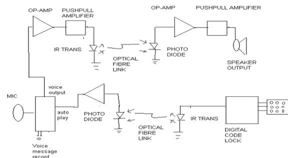
Fig.1 Block Diagram of OFVR
