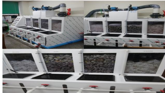
Fig. 2 Test bio-filter using the Z/M carrier layer
