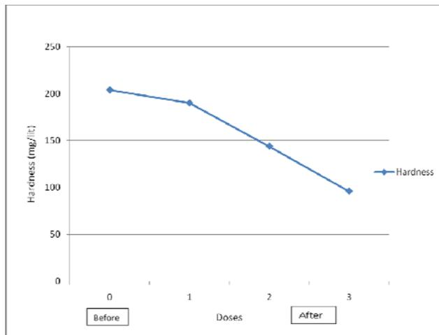
**Figure 4 : Hardness of water before and after treatment of Zia Mays seed powder.**
