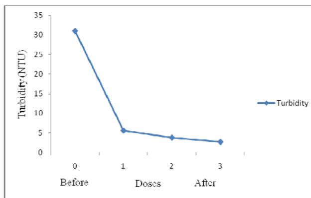
Figure 2 : Turbidity of water before and after treatment of Zia Mays seed powder.
