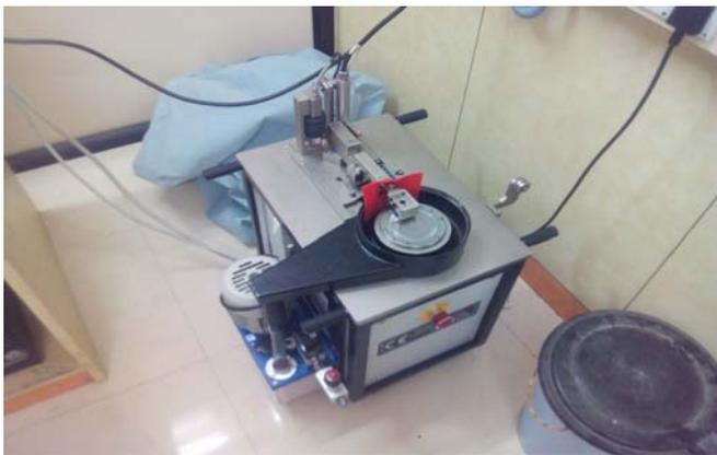
Fig. 2 : Pin on disk setup
