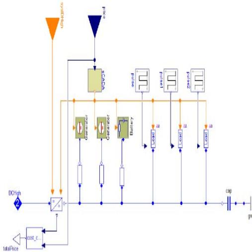
Fig. 2. Overview of an typical Modelica model of a smart house with two generators, one battery, one external connector and three loads.
