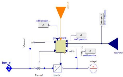
Fig. 3. Overall model of a generic generator
