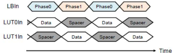
**Figure 4: Time chart of an LEDR-FPDR converter and LUTs.**
